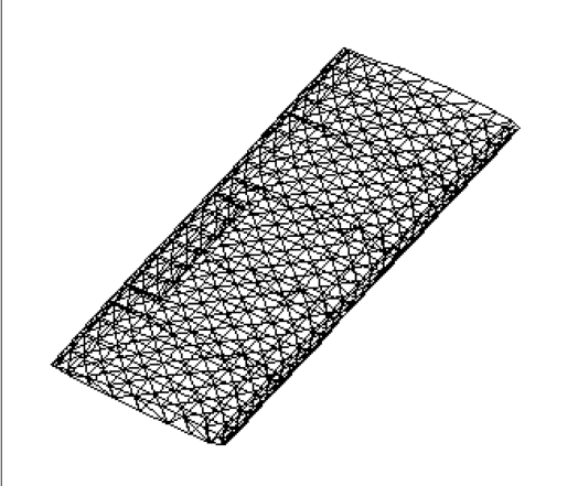
b) FE structural mesh of the wing
